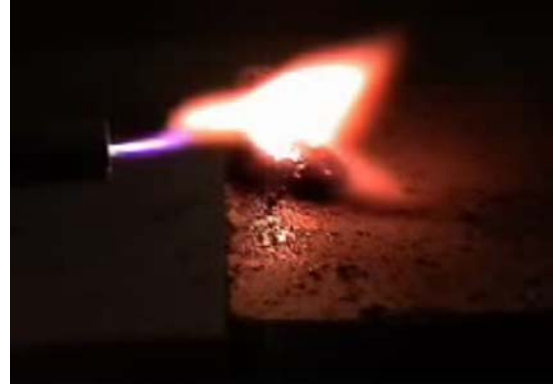
FIGURE 5. Pyrolysis of a 20-gram sample of beef tissue using the ETL EnergyBeam™ (purple/white area) technology (Sheperak, 2004).
