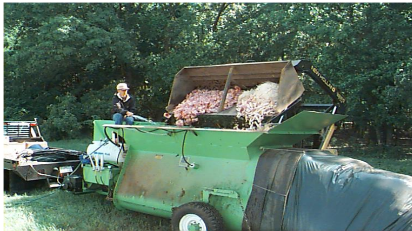
FIGURE 7. Poultry carcasses and carcass parts being added to the inlet section of an aerated synthetic tube (Cawthon, 1998).
